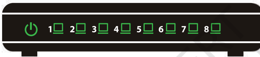
Figure 10.11: A network hub with 8 ports
